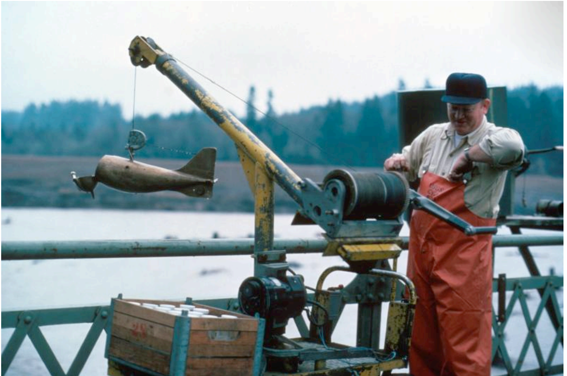
USGS suspended sediment sampling apparatus, Cowlitz River, Washington (1982)
