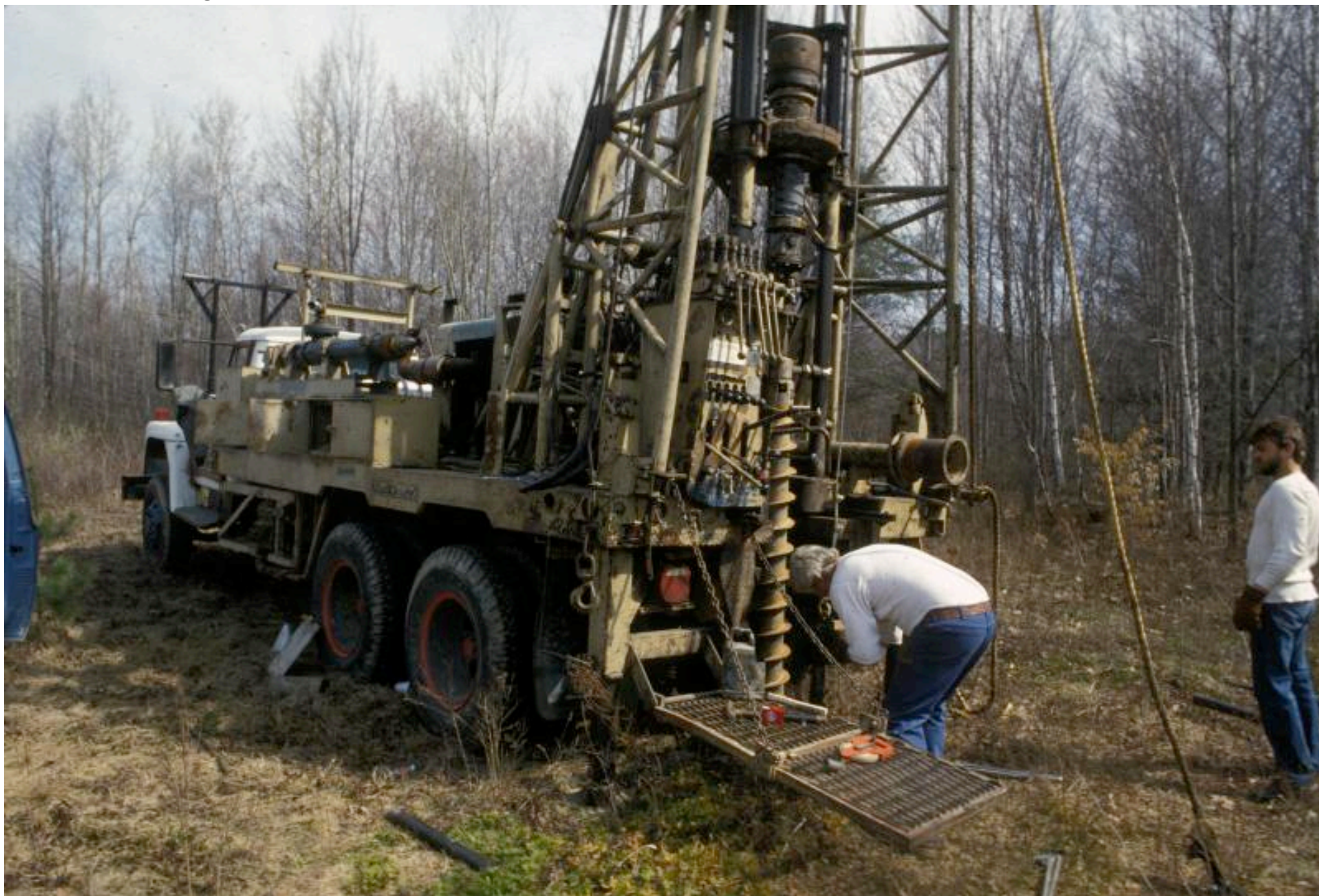
Drilling into floodplain sediments, Williamstown, Massachusetts
